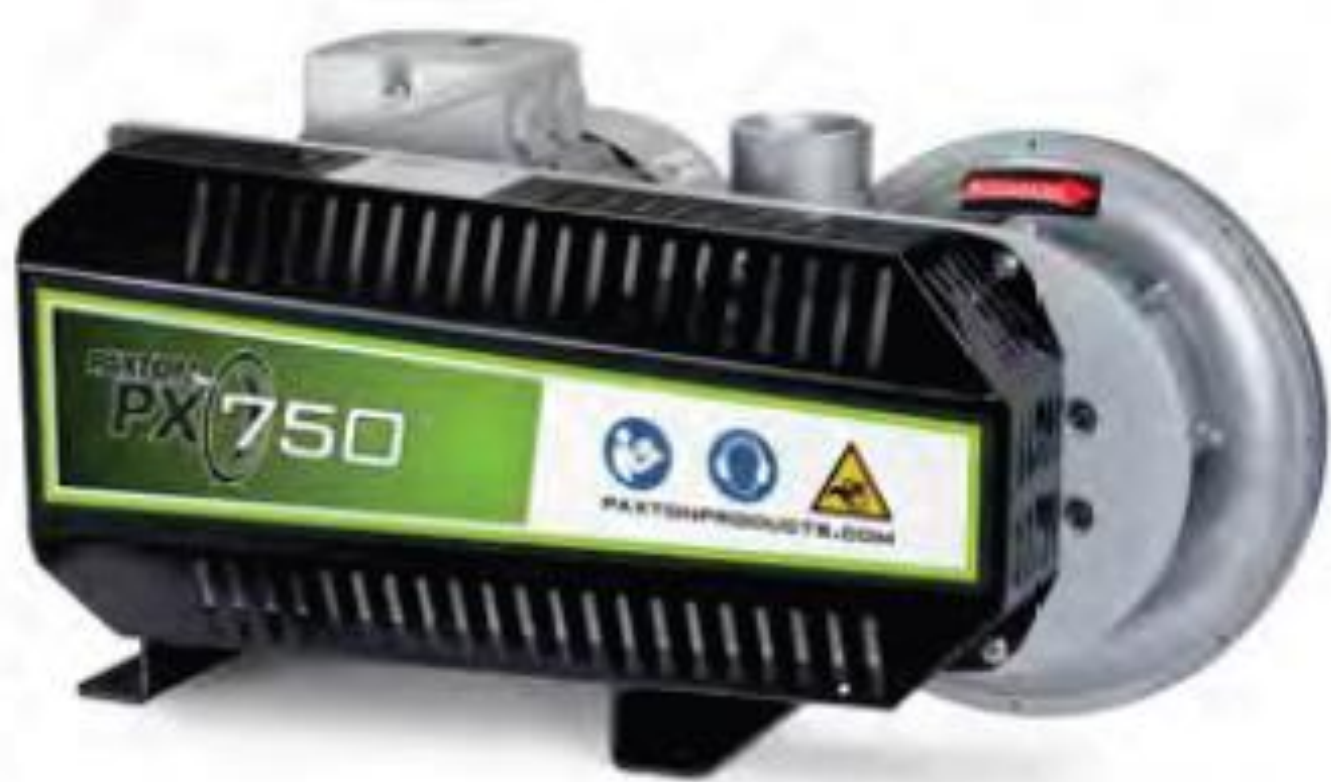
PX750 Flow Output: 1189 @ 45 (m³/hr @ mbar) 5.5kw Power Output: 170 @ 210 (m³/hr @ mbar) Outlet Diameter: 76mm
