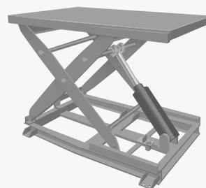
When lifting from the lowest position, electric and hydraulic cylinders push the lifter in a diagonal direction and require a large amount of power ( $1/\sin \theta$  times the lifting thrust).
