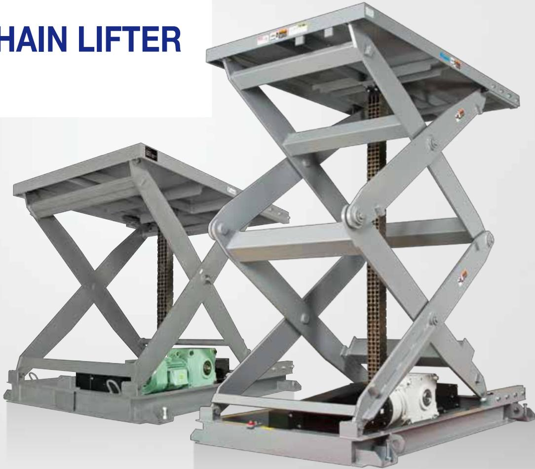
ZIP CHAIN LIFTER provides an innovative table lifter that directly transmits lifting thrust through ZIP CHAIN. It operates 3 to 10 times faster than hydraulic lifters and supports high-frequency operation, which provides energy savings as high as 50%.
