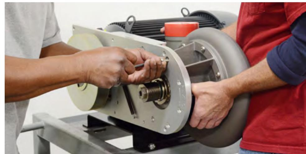
9. Slide blower pulley in through mounting plate hole to result in blower on one side of plate and pulley on opposite side. Align blower head with 8 bolts. Ensure proper alignment of outlet for existing air delivery device connections.
