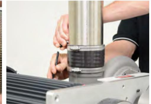
2. Remove filter and housing by loosening the coupling clamp, and pull entire housing and coupling away from blower. Set aside.
