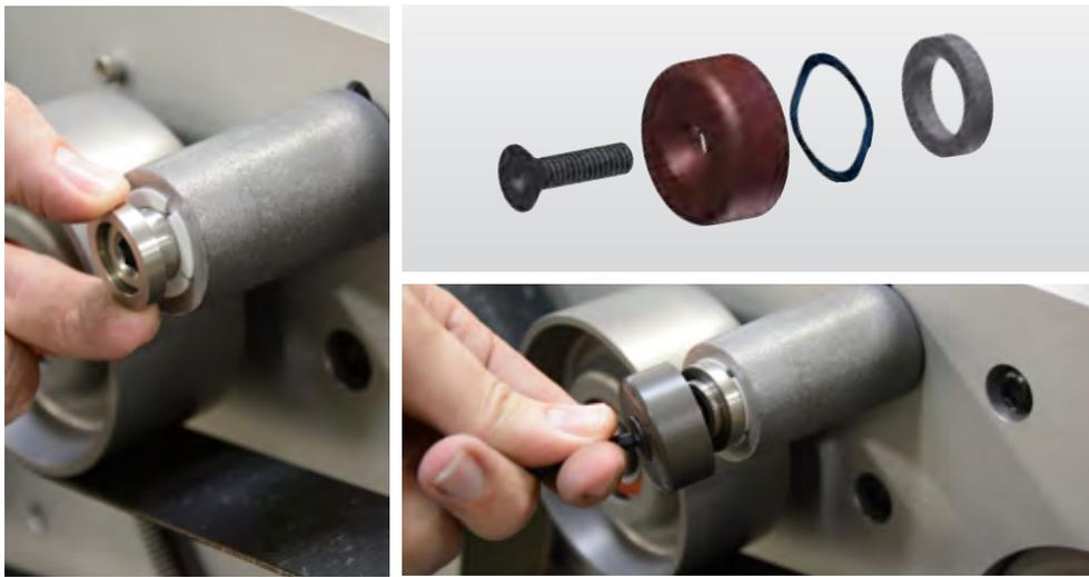
9. Put spacer on shaft then reinstall pivot arm cap, ensuring that the spring is inside cap. Tighten to 2.3 Nm (20 in-lbs) of torque.
