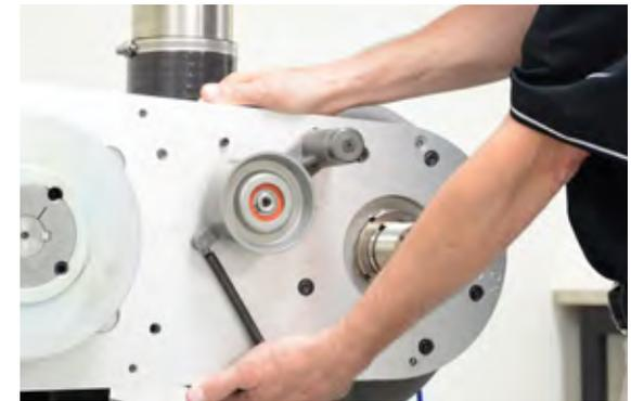
12. If it is not aligned, remove the belt and loosen the four bolts behind the motor pulley using a 3/4" wrench, and adjust the center to center distance until the tensioner is aligned.
