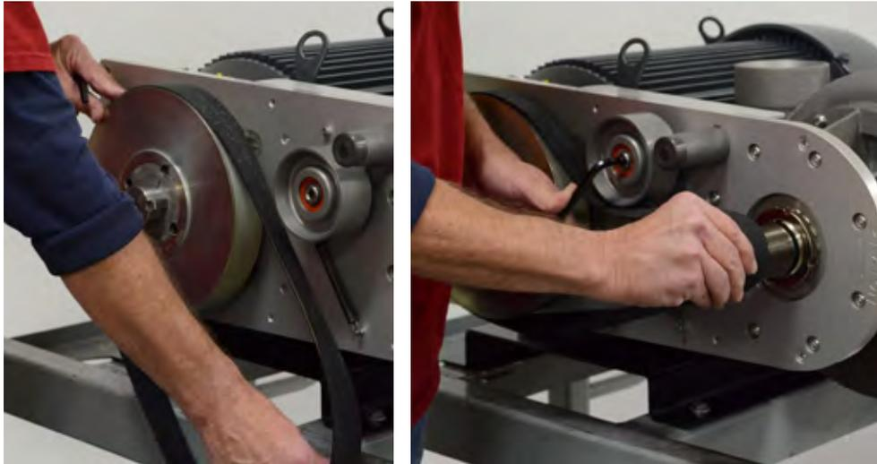
17. Using one hand to hold the belt and one to release the tension on the tensioner, wrap belt around the blower pulley ensuring that the grooves are aligned.
