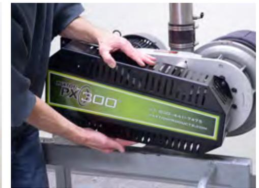
2. Remove belt guard by loosening 4 screws using T27 Torx. Place belt guard aside.
