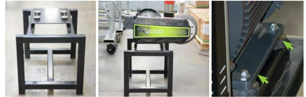
**i** The use of isolation pads under the motor plate is recommended. If needed, order **part # 8005063** from SolvAir Customer Service at **+44 1473 320 307**.
