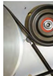
ii. If the center line of the tensioner is above the arrow, then move the motor plate to the left, which would decrease the center to center distance (moving the blower head closer to the motor pulley).
