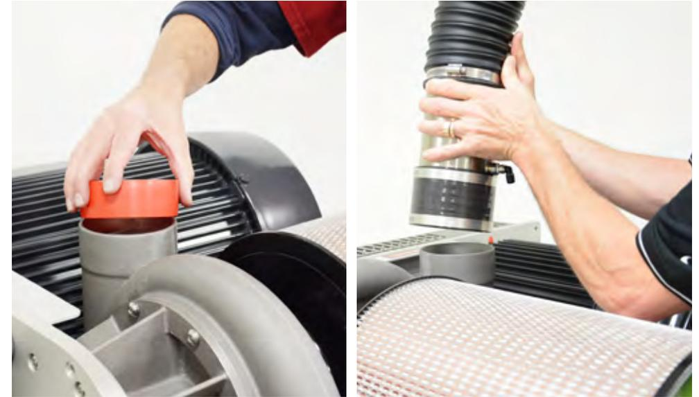
19. Reinstall hoses to blower pressure port and filter pressure port.
