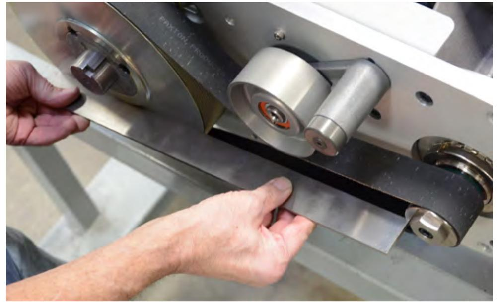
12. Check pulley alignment by using a straight edge to ensure motor pulley and blower pulley are flush to  $\pm 0.5\text{mm}$  ( $0.02''$ ).
