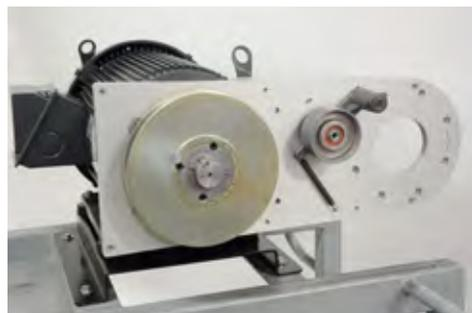
7. Using one person to steady the blower head and another to remove the bolts, slide the blower head and blower pulley away from the mounting plate.
