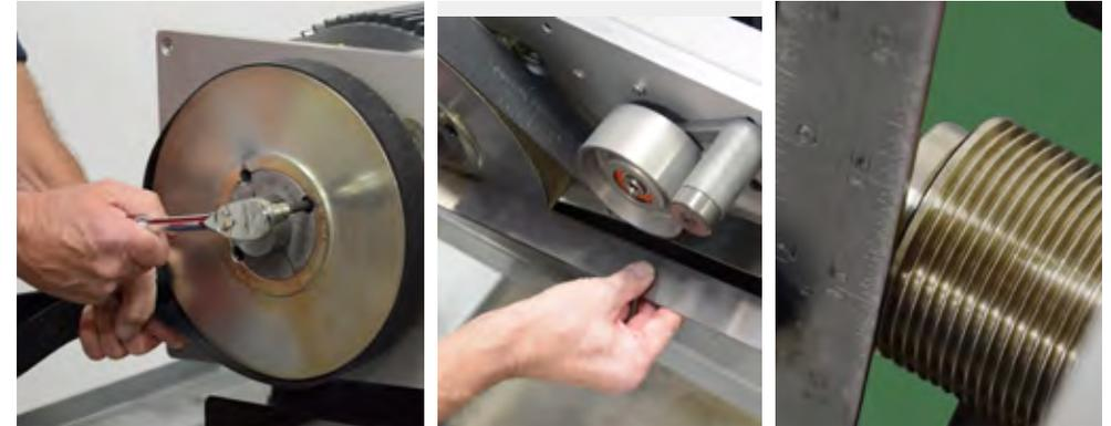
13. Using the removed bolt, put into the hole at 90 deg and tighten. When tightening the bolt into this third hole, the motor pulley will loosen so that it can be slid in or out on the shaft to cause alignment. The motor pulley should be aligned to the chamfer of the blower pulley, because tightening of the motor pulley again will draw the motor pulley out slightly, thus coming into alignment with the blower pulley.
