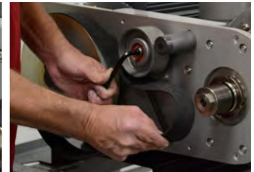
3. Using 5/16" hex key, loosen tensioner by rotating up/clockwise to release tension on belt.
