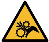
➤ **Severing/Entanglement hazard:** due to the rotating impellor - keep fingers away from the pump inlet/outlet areas.
