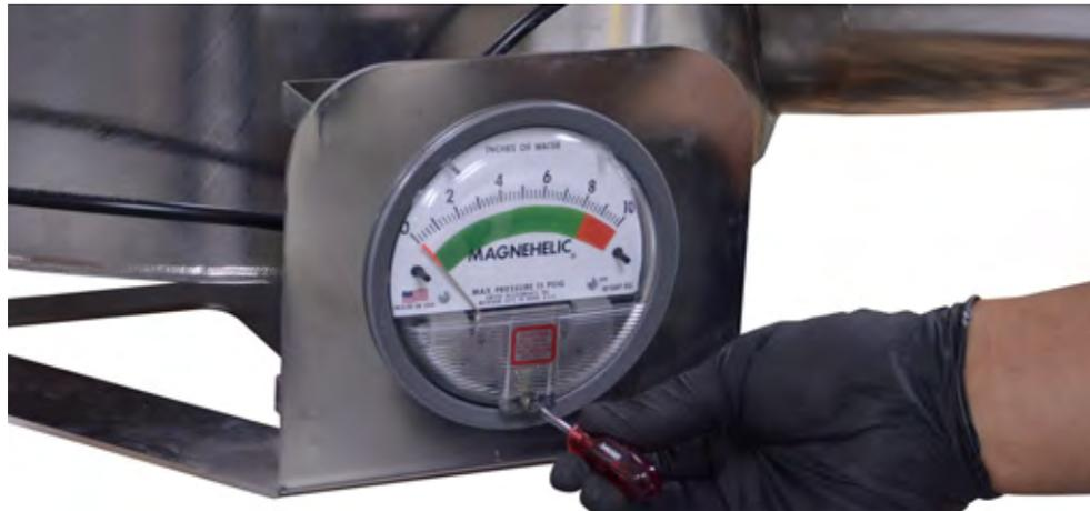
The gauge must be zeroed at startup. To zero, start the system and allow it to reach target flow rate (10–30 minutes). With the clean filter installed, and using a small flat head screw driver, adjust the gauge to read “0” cm of water column.
