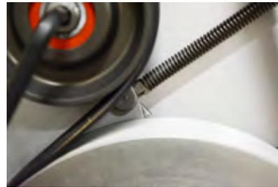
13. Once tensioner is aligned, reinstall belt and belt guard.
