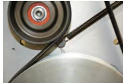
ii. If tensioner is to the left of the arrow, then decrease the center distance by moving the motor plate down (moving the blower head closer to the motor pulley)
