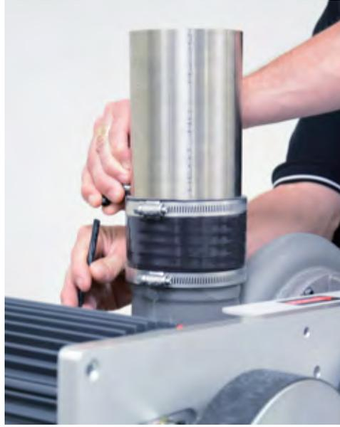
6. Remove the filter housing by loosening the screw on the clamp, then lifting the filter housing off. Place aside.
