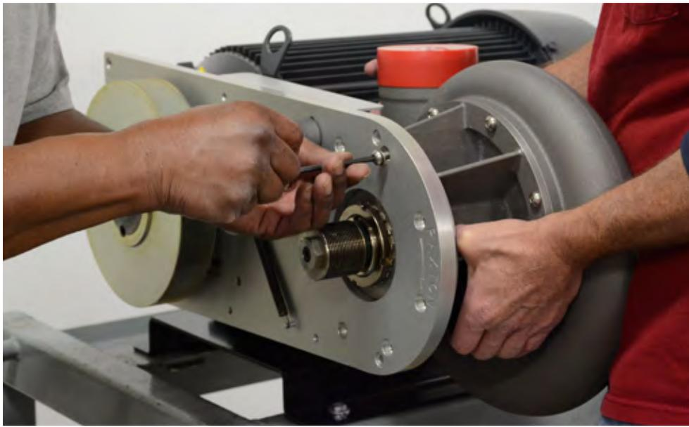
10. Finger tighten the 8 bolts, supporting the blower head on the other side of the plate.
