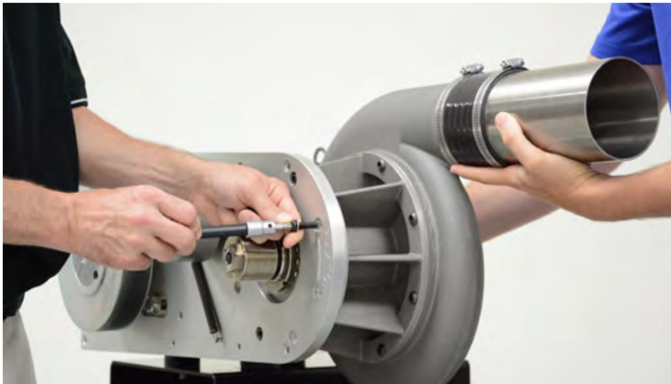
9. Rotate the blower head to the desired outlet position.
