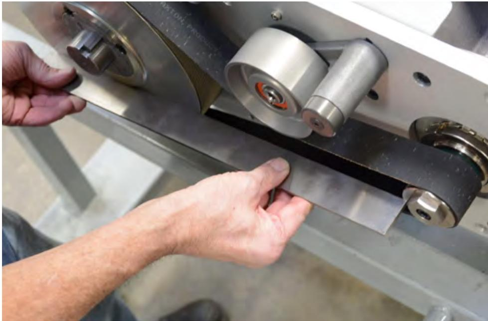
11. Check pulley alignment by using a straight edge to ensure motor pulley and blower pulley are flush to +/- 0.5mm (0.02").
