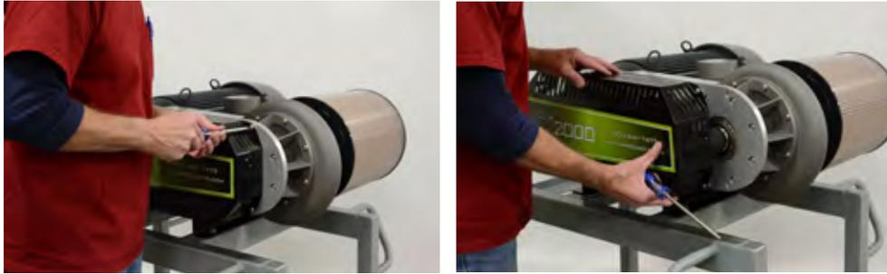
2. Remove belt guard by loosening 4 screws using T27 Torx. Place belt guard aside.
