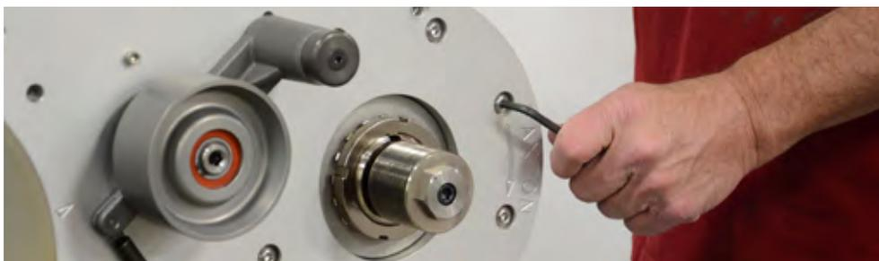
6. Using T40 Torx, loosen 8 bolts around the blower pulley that hold the blower head in place.
