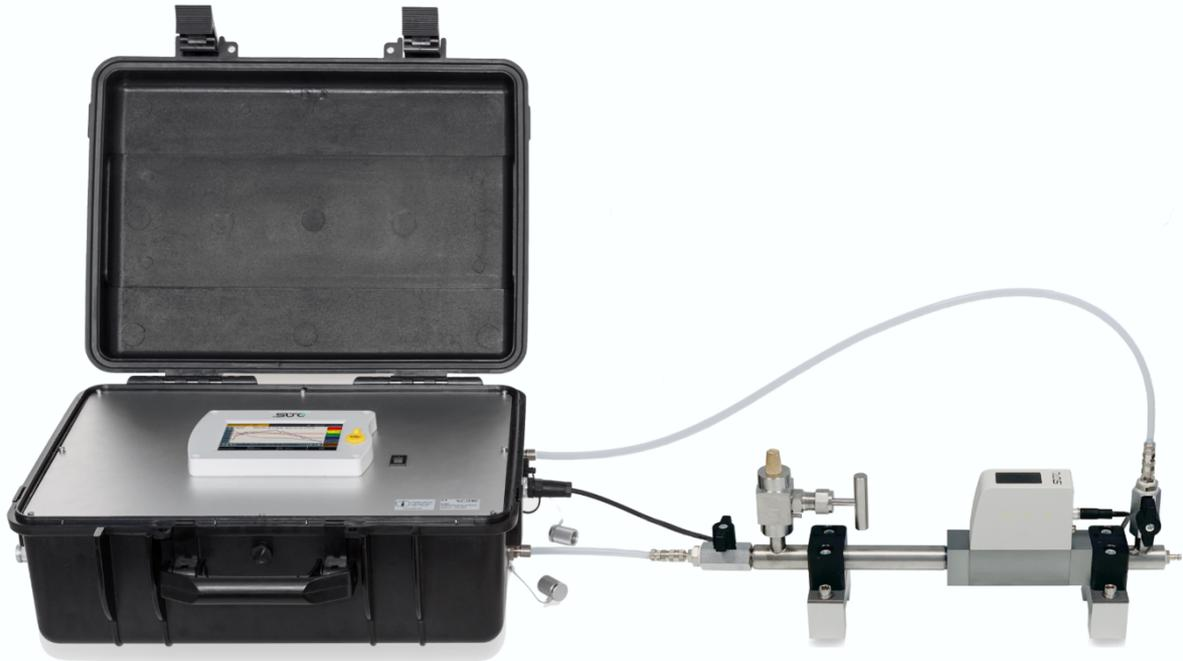
Please connect the isokinetic sampling device using the teflon hose delivered with the device. The following illustrates which outlets of the sampling device need to be connected to which inlets of the S600.
