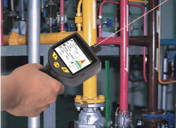
5. (Optional) Use the laser pointer to point at the leak location.
