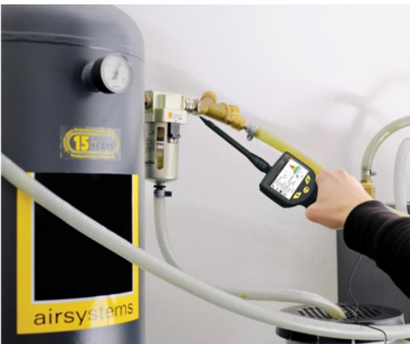
4. (Optional) If the leak point is not able to be found by using the trumpet, pinpoint the exact leak location using focus tube.
