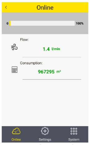
To be allowed to change settings, the App needs to scan the QR code attached on the side of the device head or on the calibration certificate. This ensures that only authorized users can access the device settings. For more information about parameter settings and operating instructions, see the S4C-FS Instruction and operation manual.
