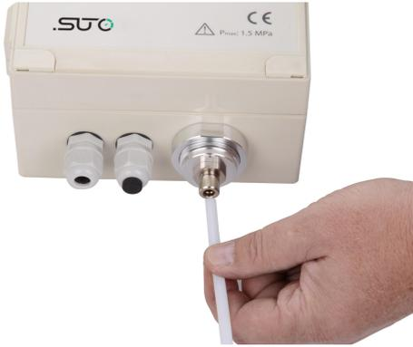
4. Connect the compressed air. The S305 will produce a small compressed air bleeding of about 2 l/min. This is required to have a good response time.
