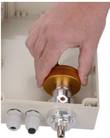
2. Screw the sensor unit out of the measuring chamber.
